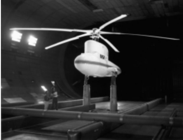
Figure 19. Sikorsky Bearingless Main Rotor (SBMR) test in NASA Ames 40- by 80-Foot Subsonic Wind Tunnel.
